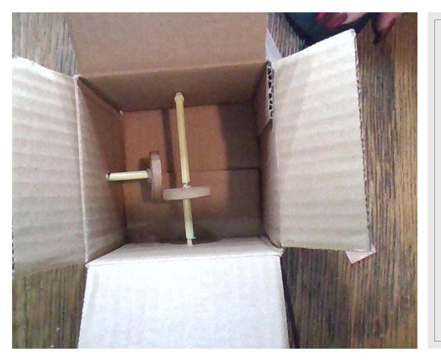
Make sure that the cam and the follower are lined up, so that when you turn the axle the follower also turns. Adjustments may be needed to get this right. (I needed to adjust a lot of times)
